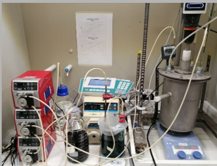
Coprecipitation is used in the synthesis of cathode precursors at the University of Oulu
